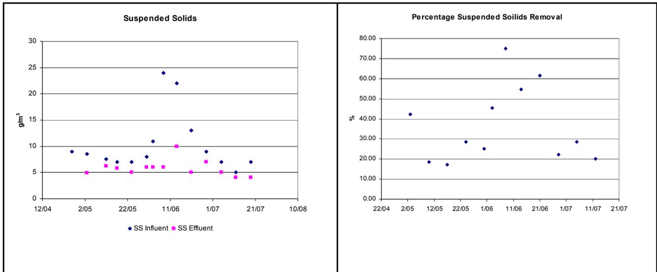
*Figure 15 Suspended solids concentrations in influent and effluent; and percent solids removed from influent by the harvester.*
