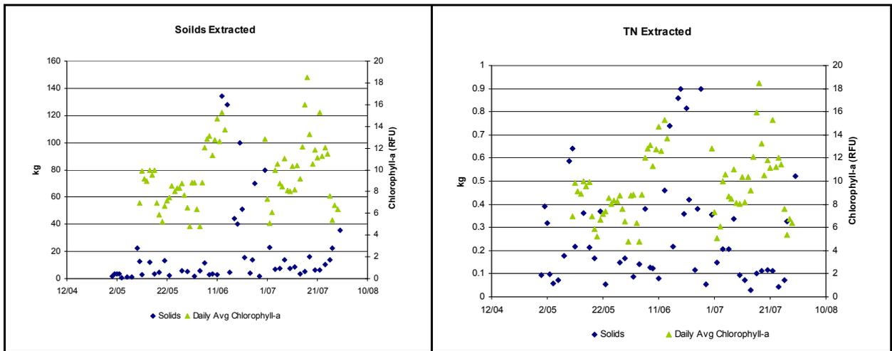
Figure 9 Weight of solids and TN extracted by harvester and Ōhau Channel chlorophyll-a daily average concentrations (by fluorescence).
