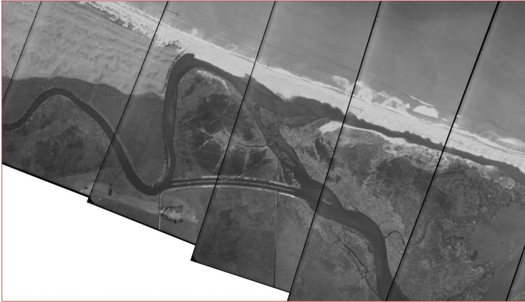
Figure 1: Aerial photograph of Te Tumu area in 1939. Note the extensive wetlands in the upper estuary, the sand dune ridge between Kaituna River and the ocean (devoid of vegetation as a result of recent river mouth migration and erosion), and “Ford’s Twin Cuts” constructed by dragline in 1927.
