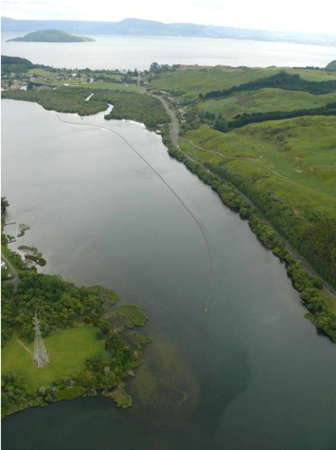
Figure 11. Photo of the Ohau Channel diversion wall, also showing Lake Rotorua (top waterbody) and including Mokoia Island (upper left). Note the variation in water appearance between in the photo foreground arising from mixing between water from the Ohau Channel from Rotoiti. Photo: Environment Bay of Plenty.
