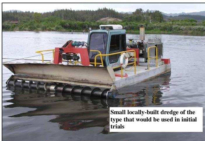
Small locally-built dredge of the type that would be used in initial trials
