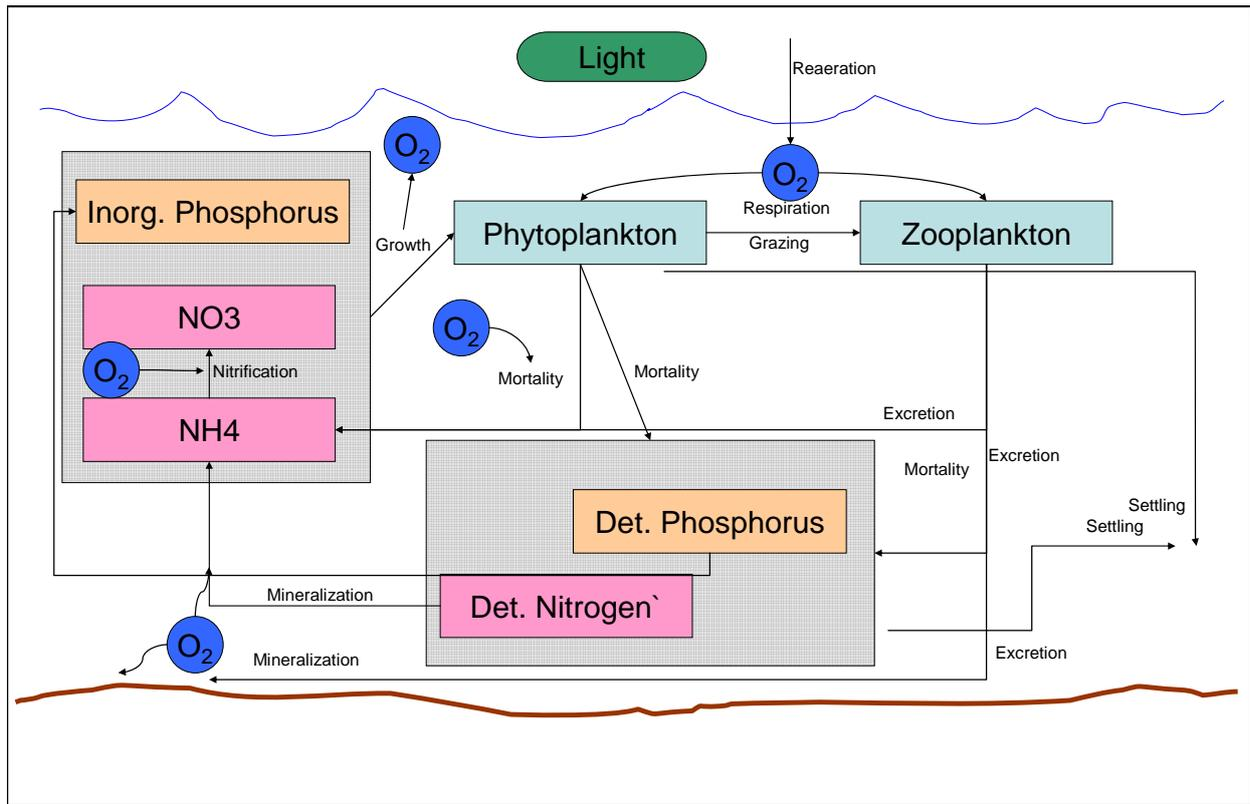
**Figure 2.1** – Simplified flow diagram of fluxes of nitrogen and phosphorus within the model 3DDLIFE.
