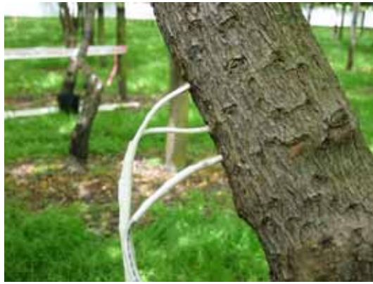
Figure 1 Heat pulse equipment installed in a kiwifruit vine.
