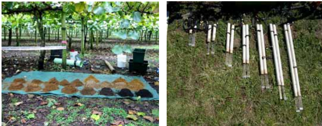
Figure 2 Installation of drainage meters (left), and Time Domain Reflectometry (TDR) probes awaiting installation (right).
