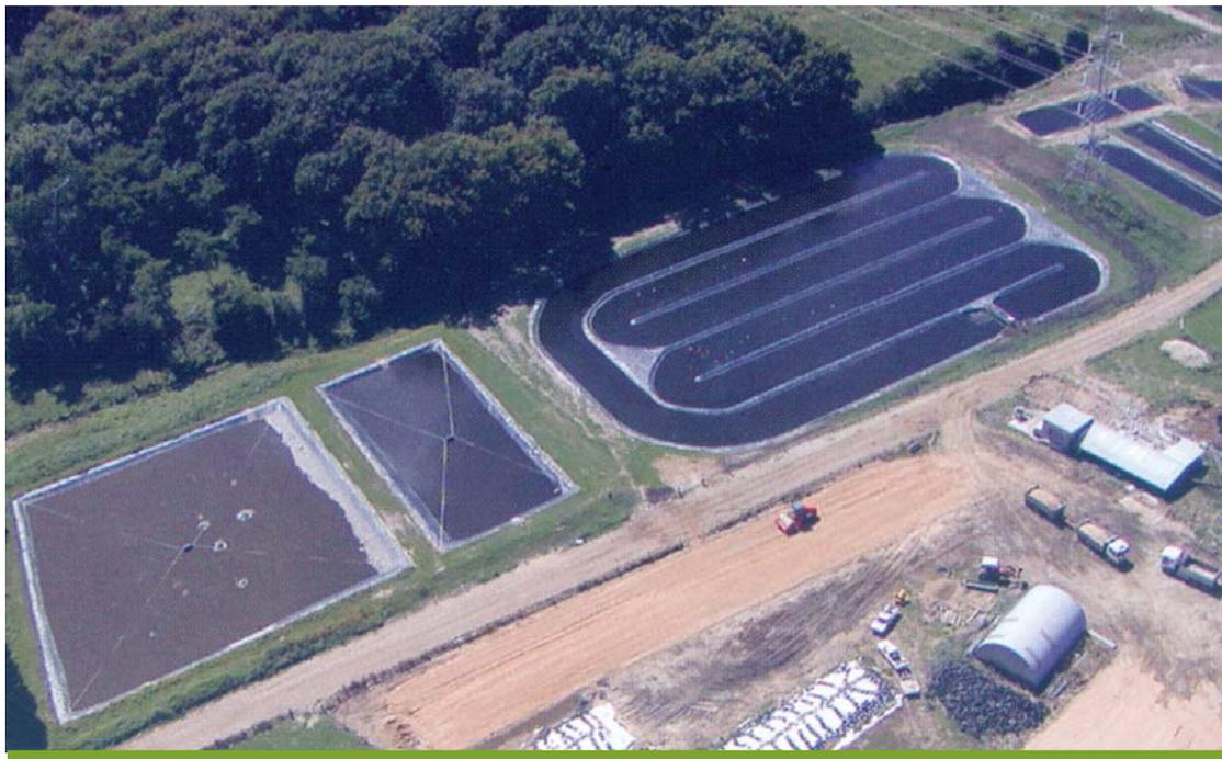
Advanced pond system trialled at NIWA (photo courtesy of NIWA)
